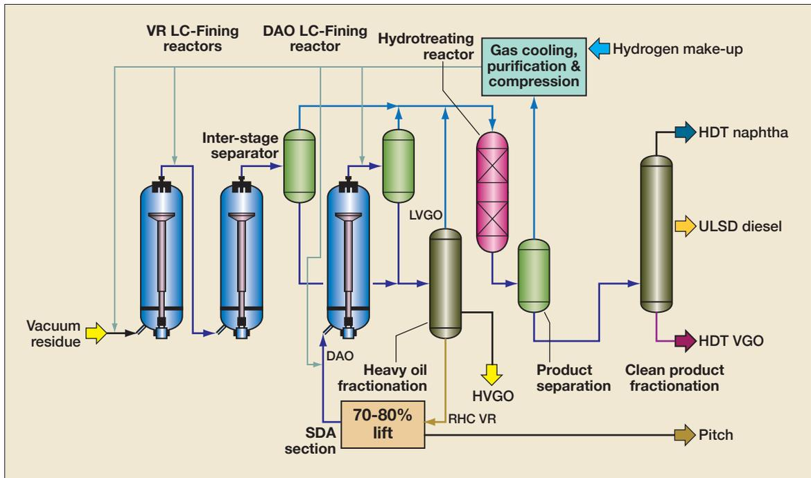
Figure 7 Schematic of the LC-Max process
