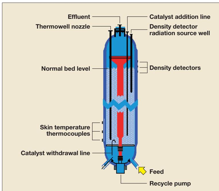
**Figure 2** LC-Fining reactor
