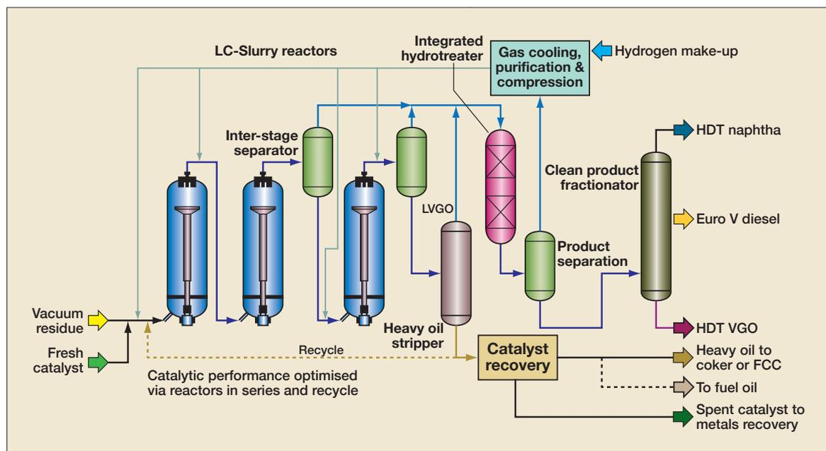
Figure 11 LC-Slurry flow scheme
