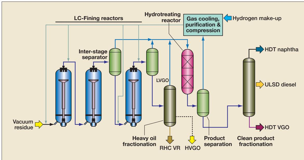
**Figure 3** Simplified LC-Fining process with integrated hydrotreating
