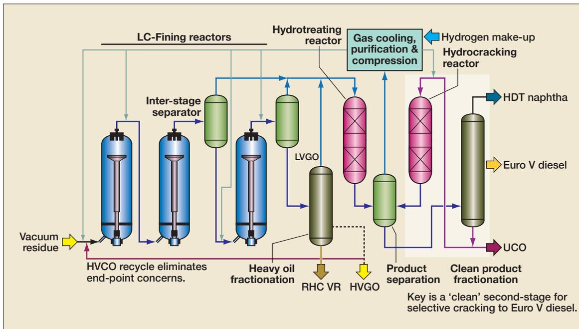
Figure 4 LC-Fining with integrated hydrocracking
