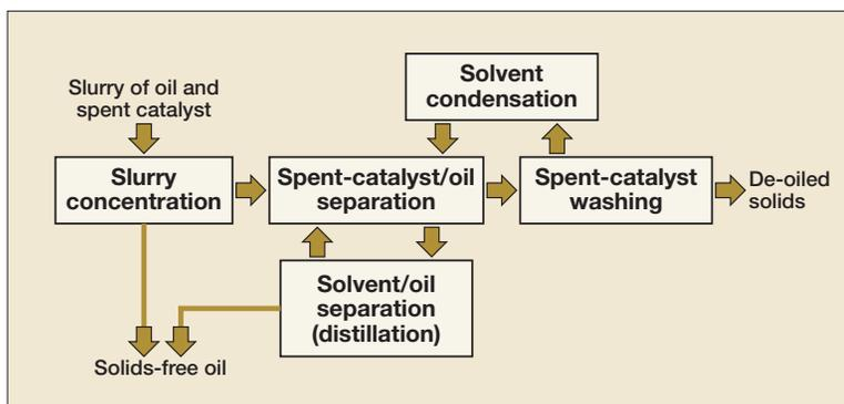
**Figure 12** LC-Slurry flow scheme
