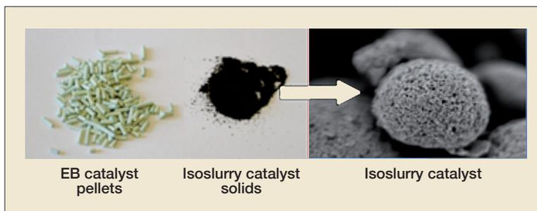
Figure 9 Isoslurry catalyst
